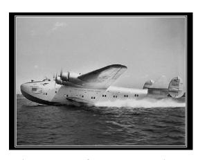
Engines: Four x 1,600 hp Wright R-2600 Twin Cyclone, 14 cylinder, air-
